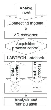
Figure 3. Block diagram of data acquisition process
