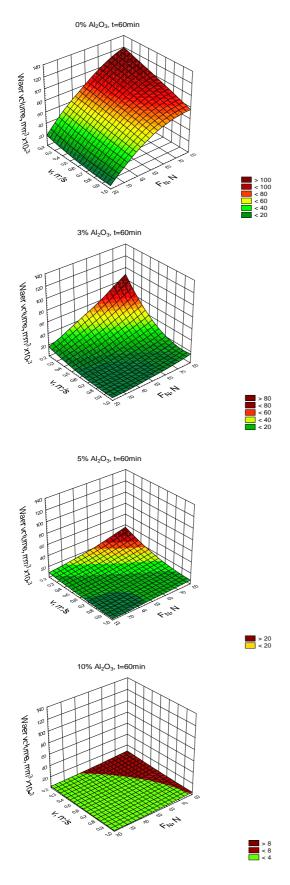
Figure 8. Relationships between wear scar width and normal load and sliding speed, for different mass weight of the reinforcements
