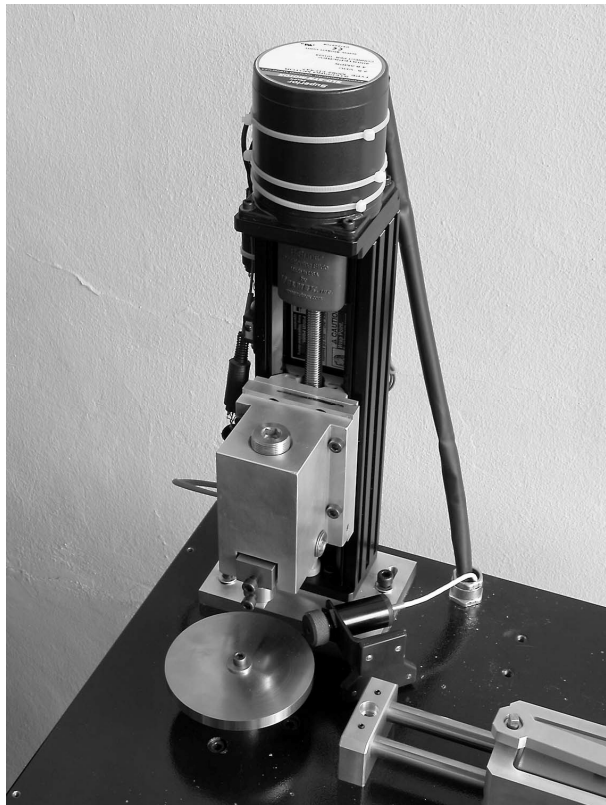
Figure 2: Unit for normal load assurance
