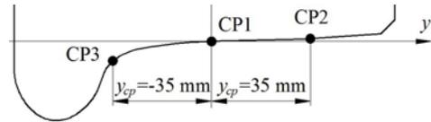
Fig. 1 Locations of wheel-rail contact point for stress-strain analysis
