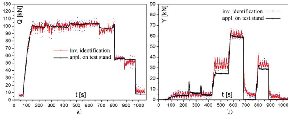
Fig. 9 Comparative diagrams of vertical force  $Q$  (a) and lateral force  $Y$  (b) applied on test stand and obtained by inverse identification
