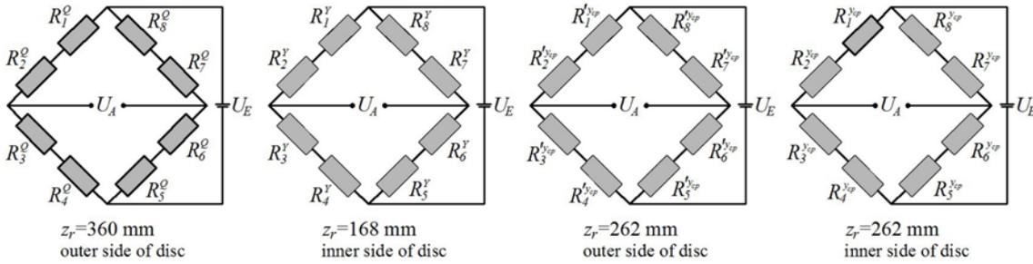
Fig. 4 Optimal way of connection of strain gauges
