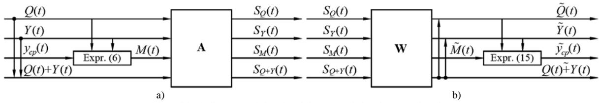
Fig. 5 Block diagrams of signals mixing (a) and signals separation (b)
