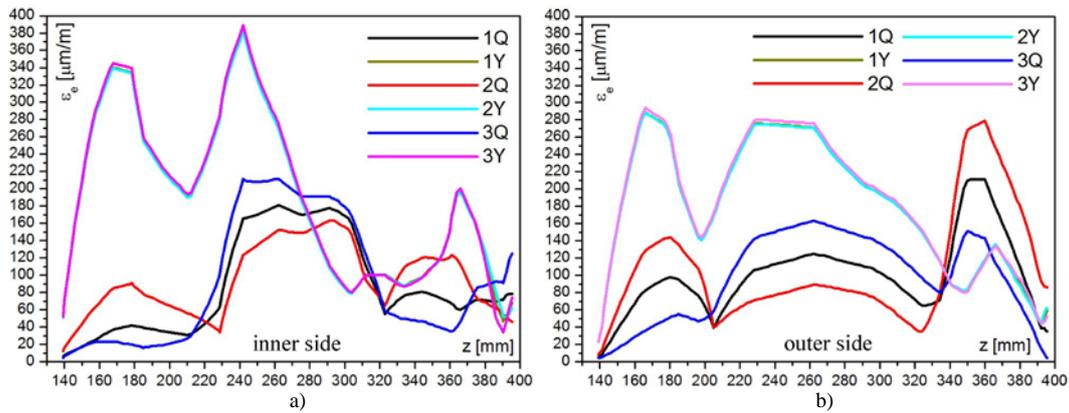
Fig. 2 Comparative diagrams of equivalent strain on inner (a) and outer side of the disc (b)
