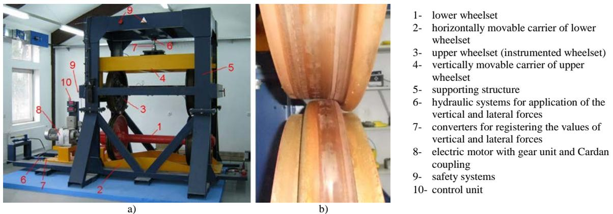
Fig. 7 Overall view of the test stand (a) and a close look at the contact point position (b)
