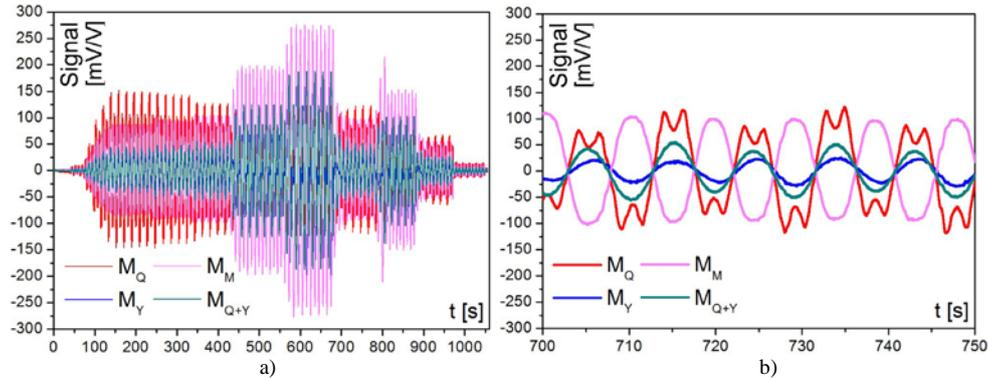
Fig. 8 Overall output signals from Whetstone bridges (a) and their parts in interval 700÷750 sec (b)
