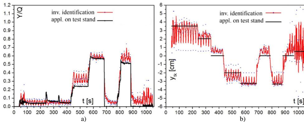
Fig. 10 Comparative diagrams of derailment coefficient  $Y/Q$  (a) and contact point position  $y_{cp}$  (b) applied on test stand and obtained by inverse identification
