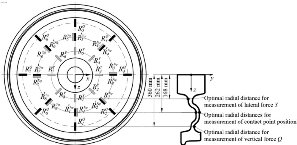
Fig. 3 Optimal radial distances, layout and number of strain gauges
