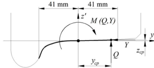
Fig. 6 Moment  $M$  of forces  $Q$  and  $Y$  in relation to the nominal contact point ( $y_{cp}=0$ )
