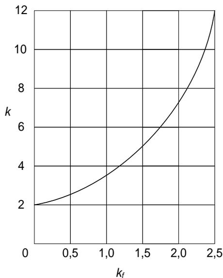
Fig. 6 The dependence of coefficient of shape  $k_f$  and coefficient of enlargement  $k$
