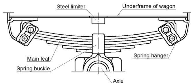
Fig. 2 Connection of leaf spring and underframe
