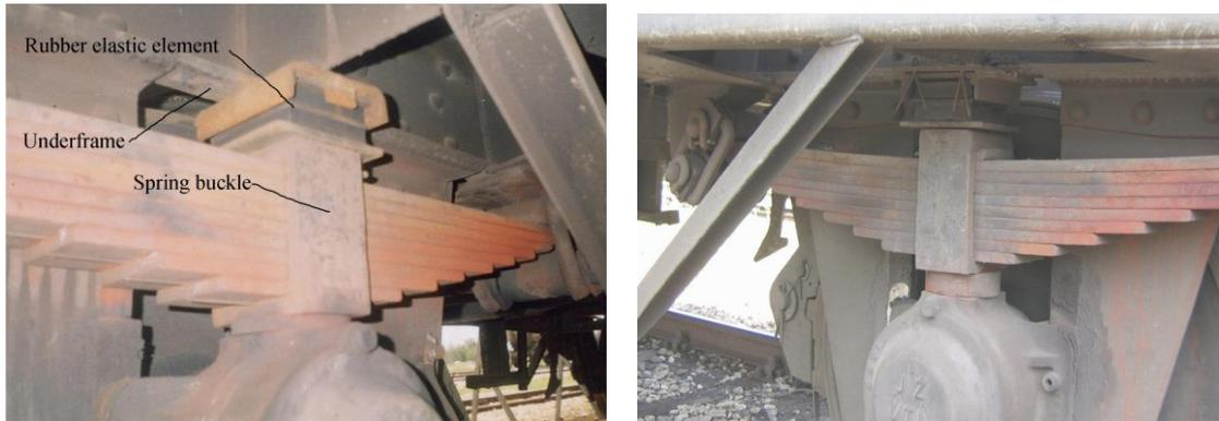
**Fig. 11 Combined suspension with leaf spring and reinforced rubber elastic element**
