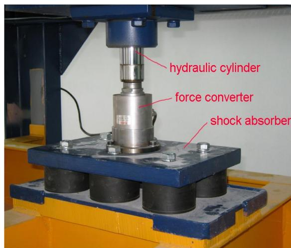
**Fig. 12 The reinforced rubber elastic elements on the test stand for calibration of instrumented wheelsets**
