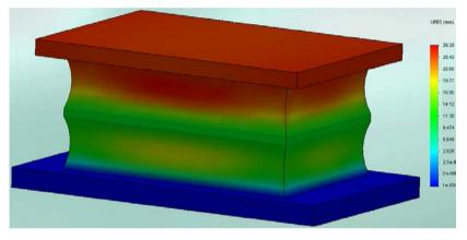
Figure 8 The deflection of rubber-metal elastic element
