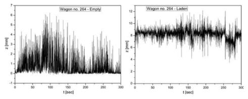
Figure 10 The measured deflection of rubber-metal element in exploitation
