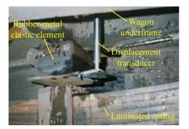
Figure 9 The exploitation tests of deflection of rubber-metal element
