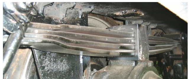
Fig. 1. The suspension of Ddam wagon for cars transportation – parabolic spring
