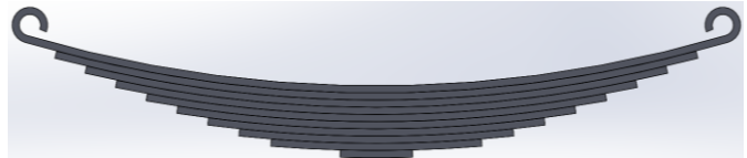
Fig. 4. The finally formed CAD model of the considered leaf spring in SolidWorks
