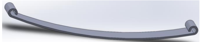
Fig. 3. The 3D geometry of main leaf formed in SolidWorks
