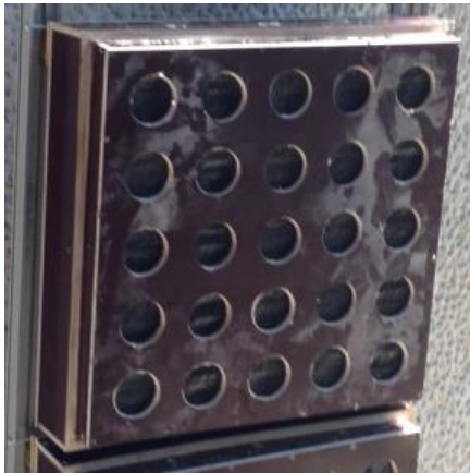
Figure 3. The modular system of the perforated box (M1).
