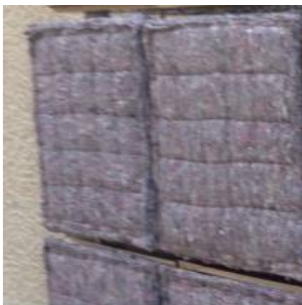
Figure 4. A modular system with a fabric backing (M2)
