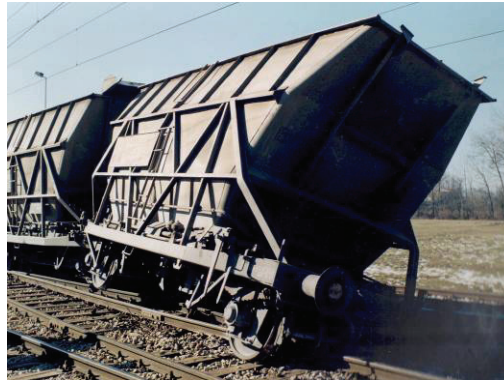
Fig. 1 The derailment of a Fbd wagon for coal transportation in the thermal power plant "Nikola Tesla" Obrenovac, Serbia
