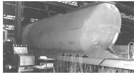
Fig. 6 Testing of supporting structure of railway vehicle [2]
