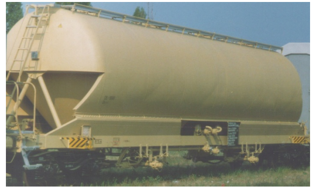
Figure 3: The wagon Uacns-z for transportation of powdered materials
