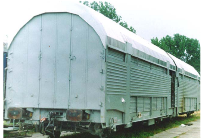
Figure 4: The wagon Hccrrs-z for transportation of cars
