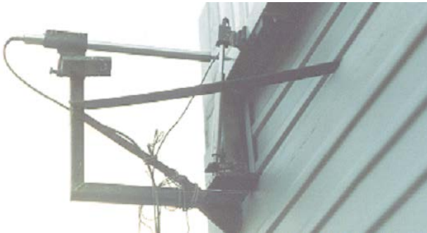
Figure 6: The testing of roof movement (wagon Hccrrss-z)
