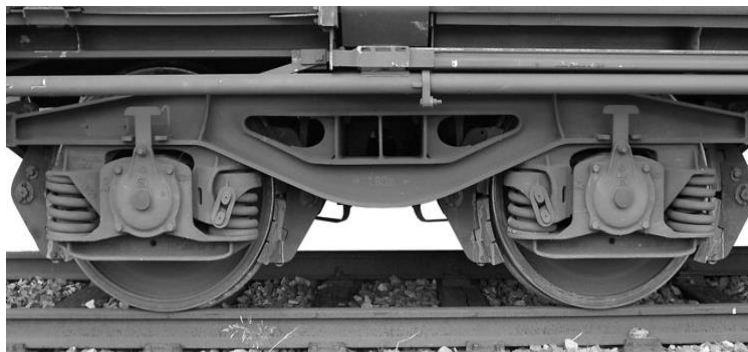
Fig. 9. Suspension of freight bogie Y25
