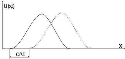
Fig. 2. Propagation of waves in the elastic continuum
