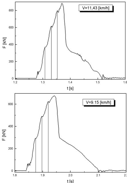
Fig. 6. Change of force on the buffers at impact of wagons
