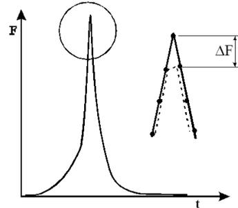
Fig. 7. Measurement of force in a collision with insufficient a frequency of acquisition
