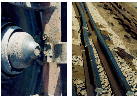
Fig.2. Typical damage of the axle and track
