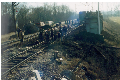
Fig.1. Derailment caused by the axle-bearing failure
