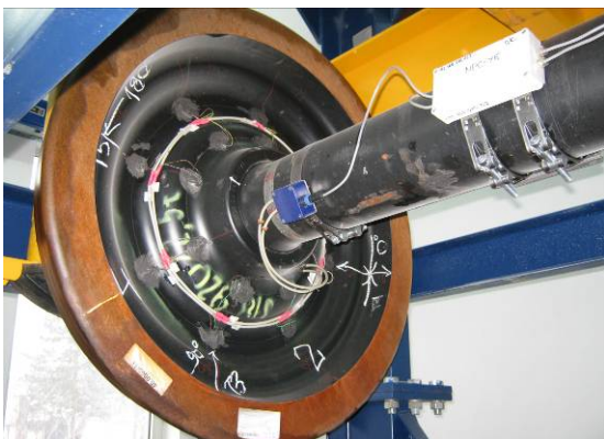
Fig. 7. The instrumented wheelset with standard monoblock wheels
