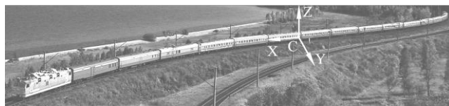
Fig.5. The train movement under the influence of its total mass and forces of traction, resistance, braking, etc.
