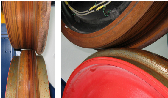
Fig.5. Wheel-rail contact on the test stand
