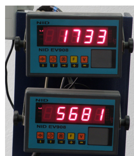
Fig.12. Alpha numeric displays for displaying the values of given forces Y and Q
