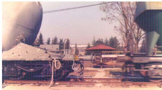
Fig.4. Two wagons impact on test polygon
