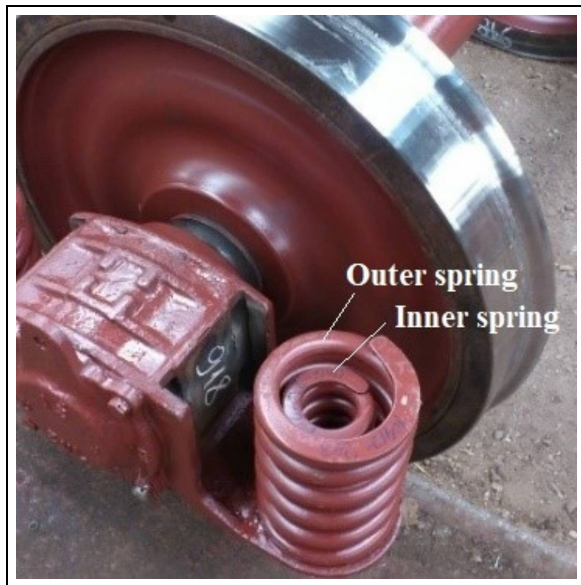
Figure 3. Set of coil springs in rail vehicles suspension.
