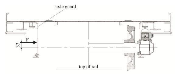
Fig. 4 Scheme of model loading; maximum lateral force for maximum stress of 345 MPa
