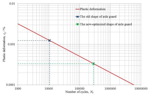
Fig. 17 Plastic strain-life curve of S355J2+N material obtained by calculation of old and new optimized shape of axle guard
