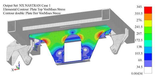
Fig. 8 Von Mises equivalent stress field - model with new optimized shape of axle guard
