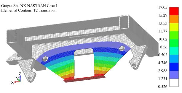
Fig. 9 Lateral displacement field  $- U_y - model$  with old shape of axle guard
