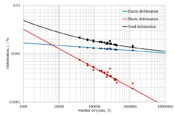
Fig. 2 Strain-life curve resulting from uniaxial tension-compression fatigue tests of S355J2+N material
