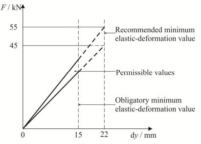
Fig. 3 Rigidity of axle guard with constant stiffness (reinforced type)
