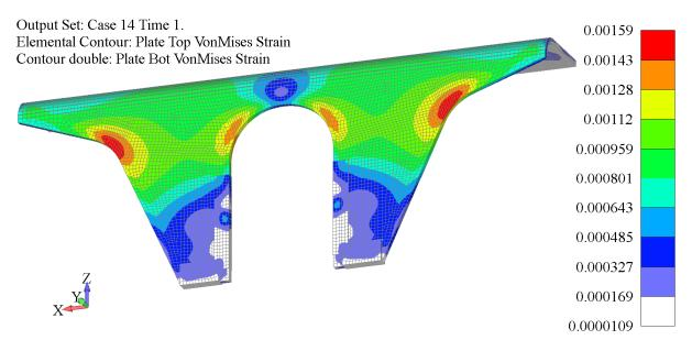
Fig. 14 Total strain field -new optimized shape of axle guard
