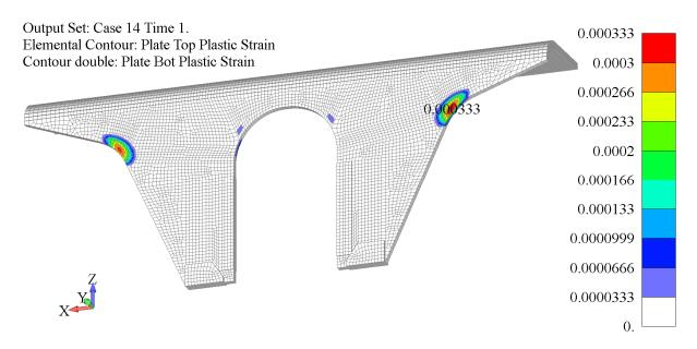
Fig. 16 Plastic strain field –new optimized shape of axle guard
