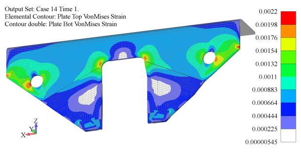
Fig. 13 Total strain field -old shape of axle guard
