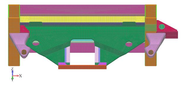
Fig. 5 3D model of running gear of Hccrrs 2x2 axle car-carrying wagon with old shape of axle guard – finite element mesh
