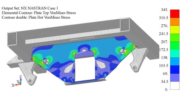
Fig. 7 Von Mises equivalent stress field - model with old shape of axle guard
