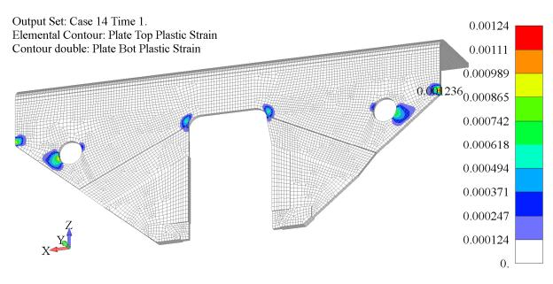
Fig. 15 Plastic strain field -old shape of axle guard
