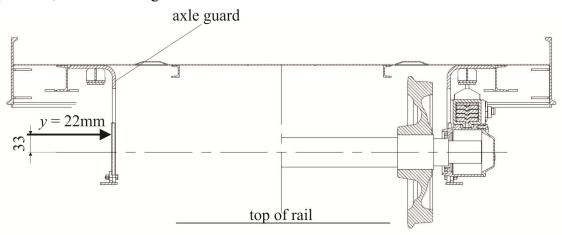
Fig. 12 Scheme of model loading; maximum lateral displacement y = 22 mm
