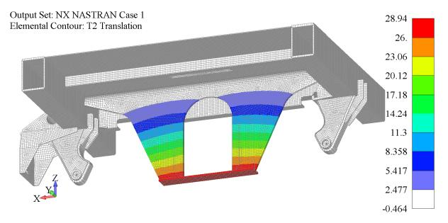
Fig. 10 Lateral displacement field  $-U_y$  - model with new optimized shape of axle guard
