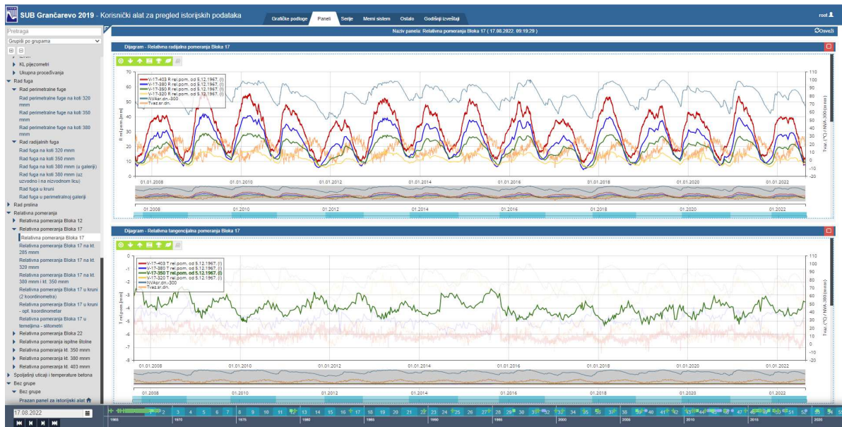
Figure 6. The relative displacement of the central Block 17 in the radial and tangential directions
