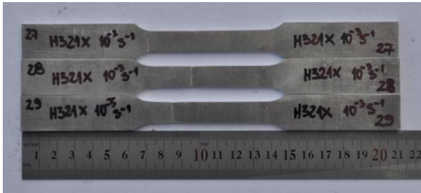
Fig. 2. Three flat AA5083-H321 specimens after uniaxial tensile tests.
