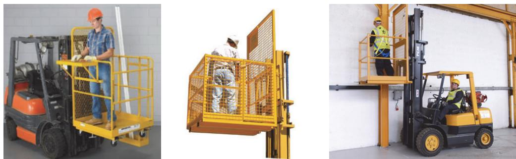
Fig. 2 Examples of correct use of work platforms on forklift trucks
