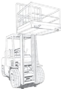
**Fig. 3 Forklift truck with non-integrated working platform**
