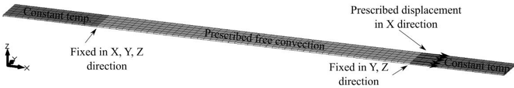
Fig. 1. Finite element mesh with loading and boundary conditions (Dunić et al. 2014)
