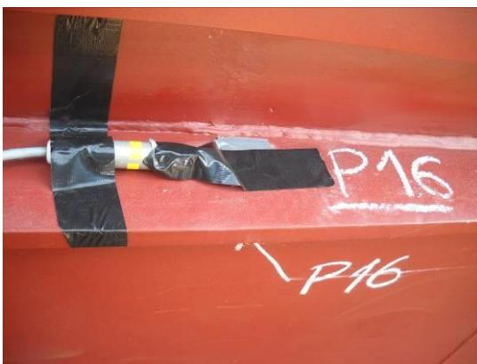
*Figure 8: Strain gauge P16*
