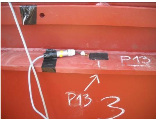
*Figure 9: Strain gauge P13*
