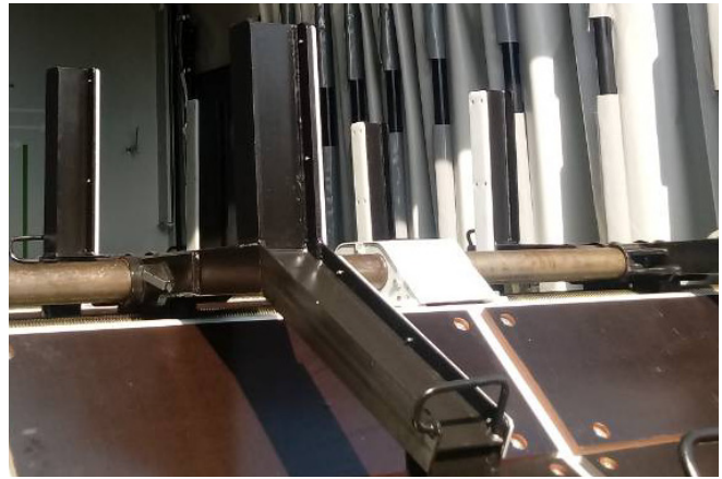
Fig. 3. Securing arm on Shimmns wagon
