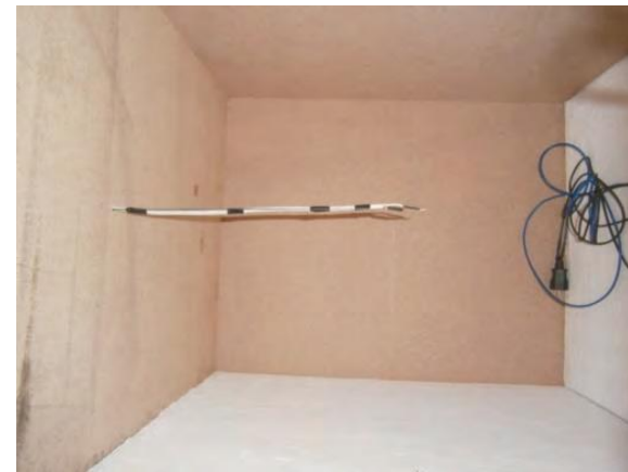
Figure 4. The interior of the test model – show the position of the PT100 probe
