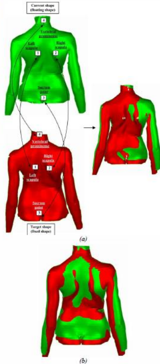
Fig.6. Local registration for 3D polygonal back shape scan data (source and target shapes) using 4 anatomical reference points (a) matching (b) registration
