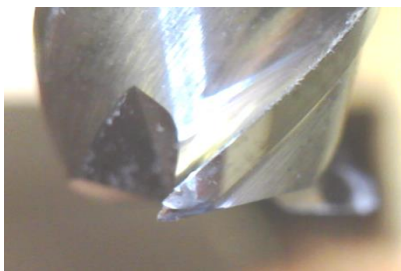
Figure 8. A worn tooth of the tool
