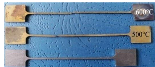
Figure 3. Specimens before and after fracture at temperatures of 500 °C and 600 °C
