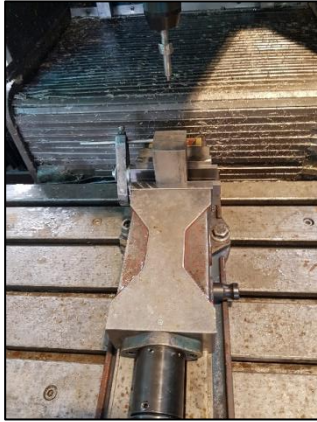
Figure 14. Clamping of work piece
