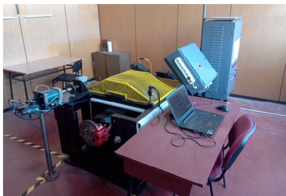
Fig. 2. Inertial brake dynamometer Brake Dyno 2020
