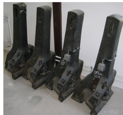
Figure 19: Sets of measuring automatic couplings SA-3 with strain gauges installed
