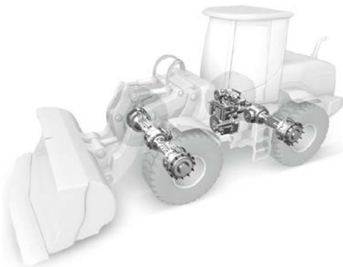
Figure 16: Generator-electric motor gearbox type [10]
