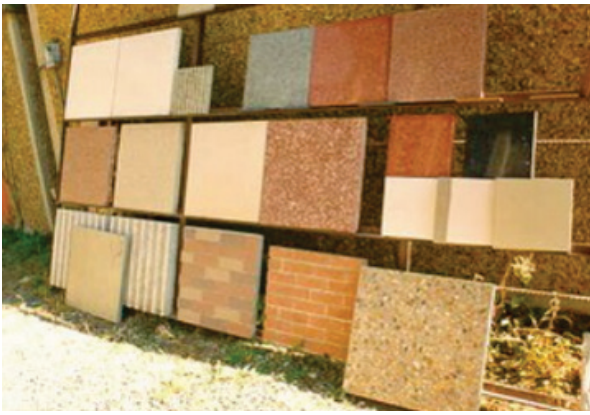
Figure 2. Surface treatment textures of barriers [1]
