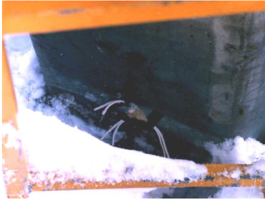
Fig. 10. Measuring poin , strain gauges
