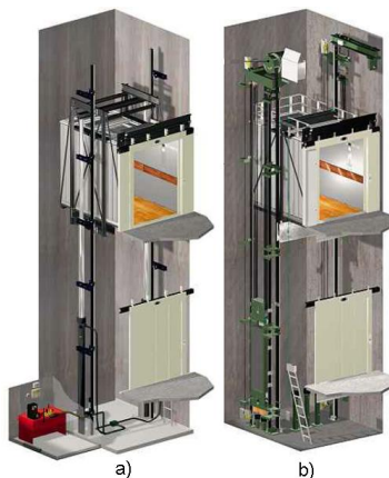
Fig. 1. The most common elevator drive types a) pushing up from below by hydrocylinders b) pulling up from above by electric drive and traction cables
