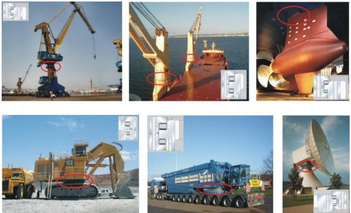
Fig. 2. Examples of top and bottom building revolving bond use with various machines
