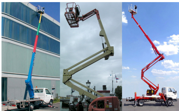
Fig. 1. MEWP boom types: telescopic, articulating and combined boom type
