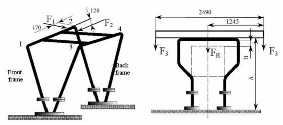
Fig. 2. Loads of protective frame
