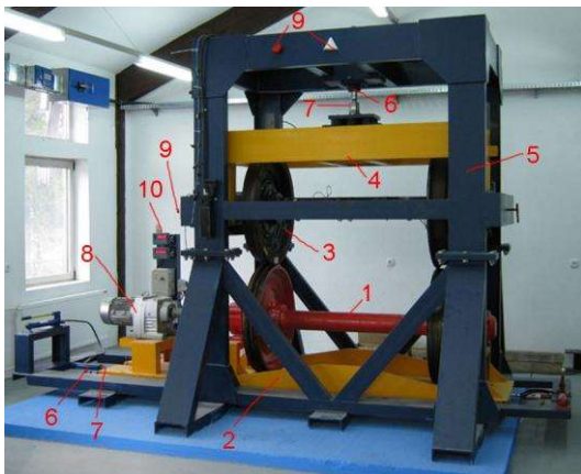
Fig. 3. Device for calibrating and testing measuring axial structures of the cars
