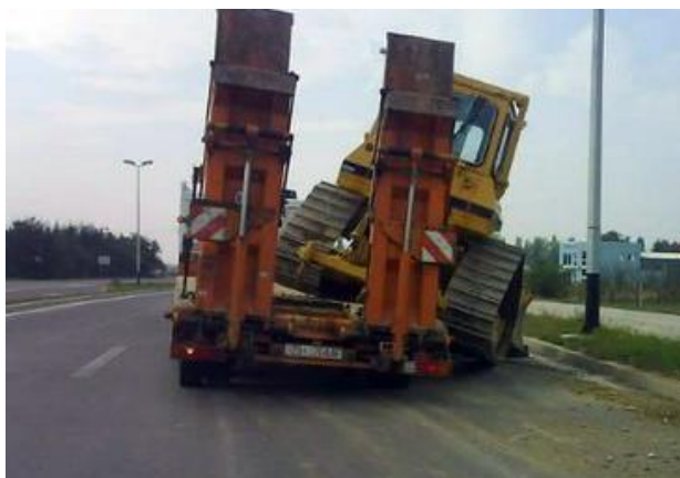
Fig.1 Construction machine slips off the trailer
