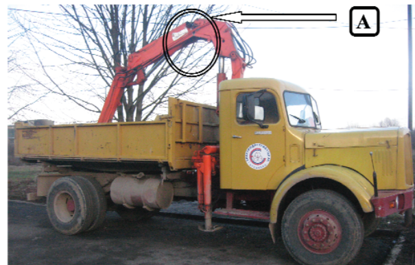
Figure 2. Point of the fracture initiation in the crane Atlas 3006
