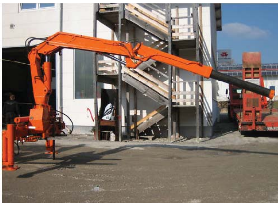
Figure 1. Hydraulic truck crane Atlas 3006
