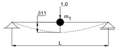
**Picture 3.** The model of oscillation of the main girder with concentrated mass
