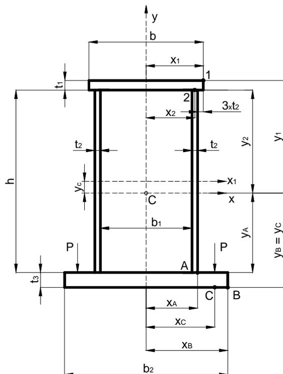
Picture 1. The box section of the single-girder bridge crane
