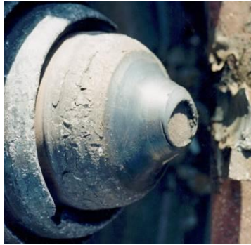
Fig. 5. Failure of axle-bearing
