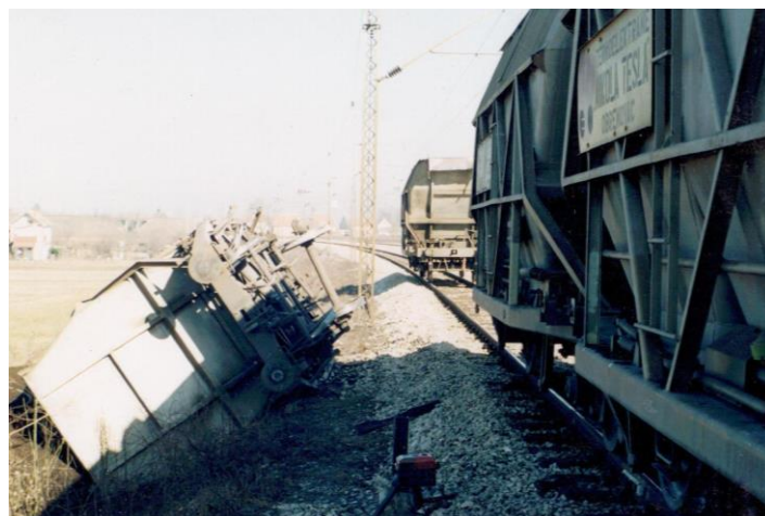
Fig. 4. Derailment of wagons for coal transportation
