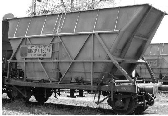
Fig. 1. Fbd wagon for transporting coal
