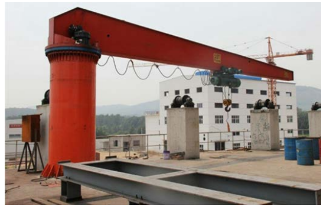
Figure 1: Heavy-duty column-mounted jib crane with a non-uniform boom [15]
