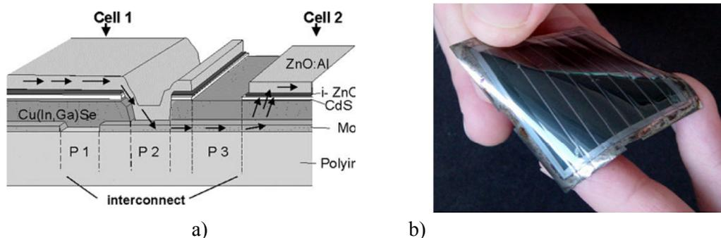
Fig. 7. a) Patterning scheme for monolithic cell integration on a polyimide substrate
