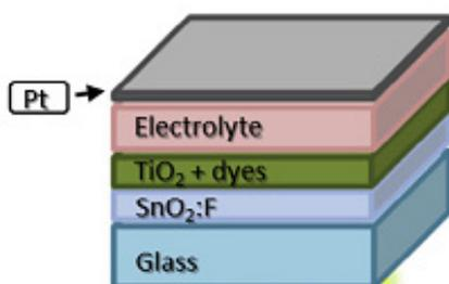
Fig. 6 Solar cell device based on DSSC
