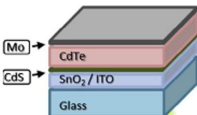
Fig. 3 Solar cell device based on CdTe
