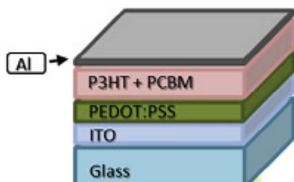
Fig. 5 Solar cell device based on OPV
