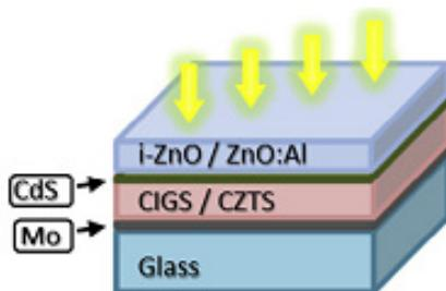
Fig. 4 Solar cell device based on CIGS/CZTS
