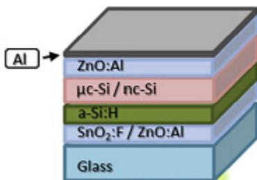
Fig. 2. Solar cell device based on a-Si/ $\mu\text{-Si}$
