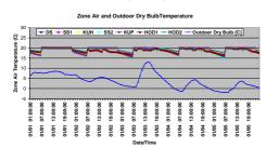
Figure 4 – Outdoor dry bulb temperature and air temperatures calculated by EnergyPlus from January 1<sup>st</sup>-5<sup>th</sup>
