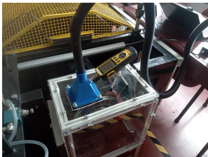
Figure 3. Device for measuring the concentration of particles mounted on the housing.
