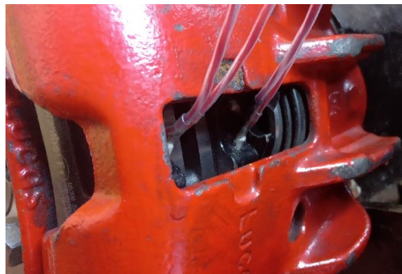
Figure 2. Temperature sensors for measuring the brake pad temperature.
