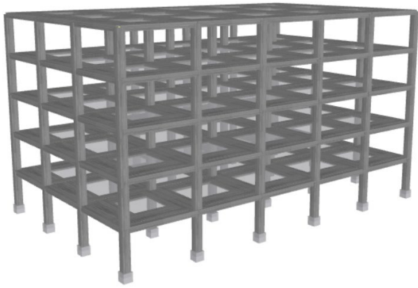
Figure 1. 3D model of the structure in SeismoStruct
